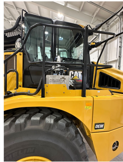
Custom Bolt on bracket designed to fit specifically on this unit
